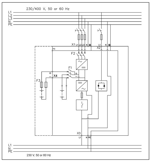
Figure 8 Wiring diagram of UPS N-model.
